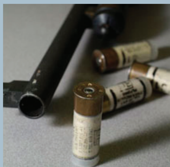
>> The bean bag gun fires cartridges filled with tiny bags of sand.
