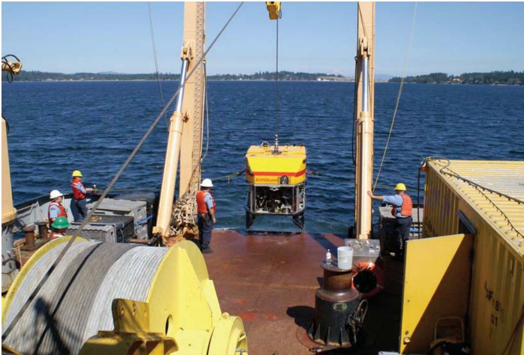
Figure 11. Deploying ROPOS prior to dropping pig carcass, for ROPOS to place carcass at camera site.
