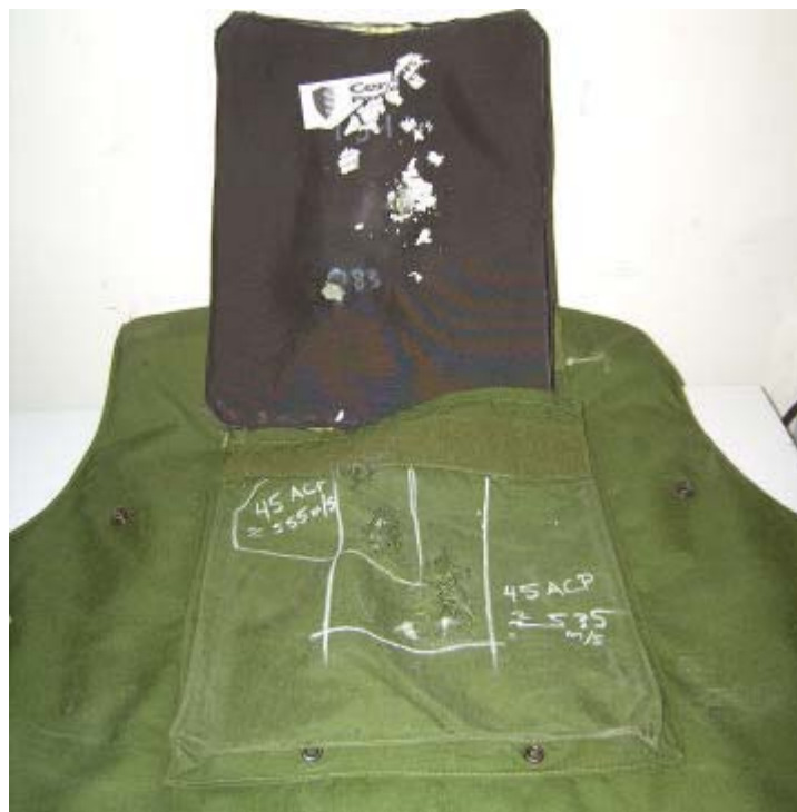
Figure 32: View of Hard Armour Tested with .45 Caliber Bullets
