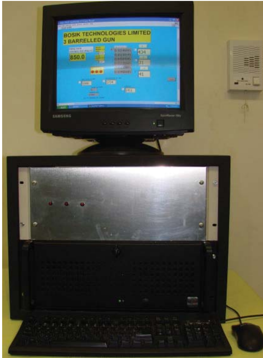
Figure 2: Computer Controls for Setting Firing Rate and Measuring Speed
