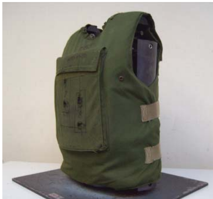
Figure 5: Complete Target Vest over Foam and Mannequin
