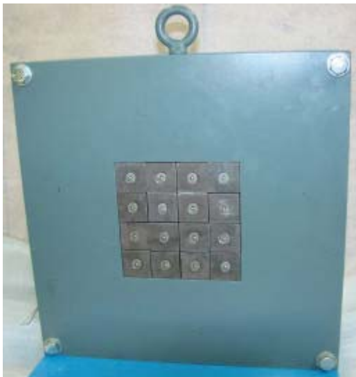
Figure 11: Front View of Instrumented Plate with 16 Load Cells and the Designation of the Load Cells
