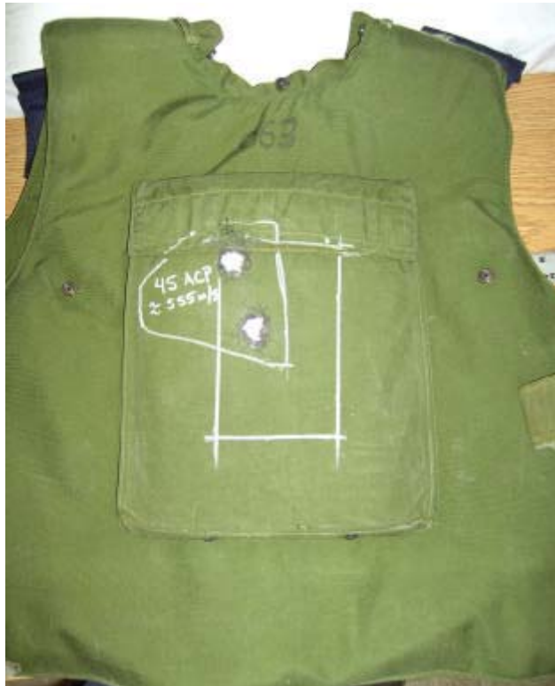
Figure 31: Sample Undergone .45 Caliber Testing (exterior)
