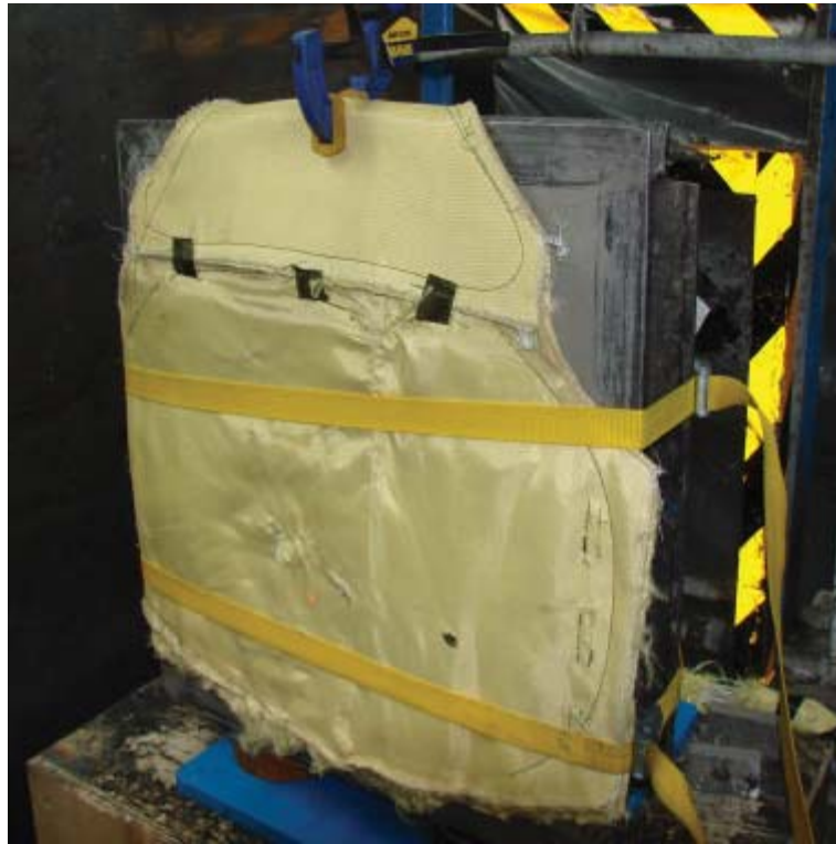
Figure 12: Set Up For Determining V-50 Penetration Velocities with Clay Backing
