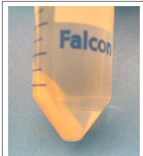
Figure 5: “Clarification” of huma saliva prior to testing. After freezing and thawing, precipitate is removed by centrifugation and supernatant decanted for device testing
