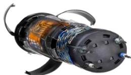
XREP Projectile, with stabilizing fins and electrodes deployed after launch
