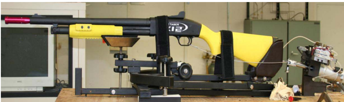
All fired rounds were fired using a computer controlled, laser-sighted X12 in a gun vise. (From Bir brief)
