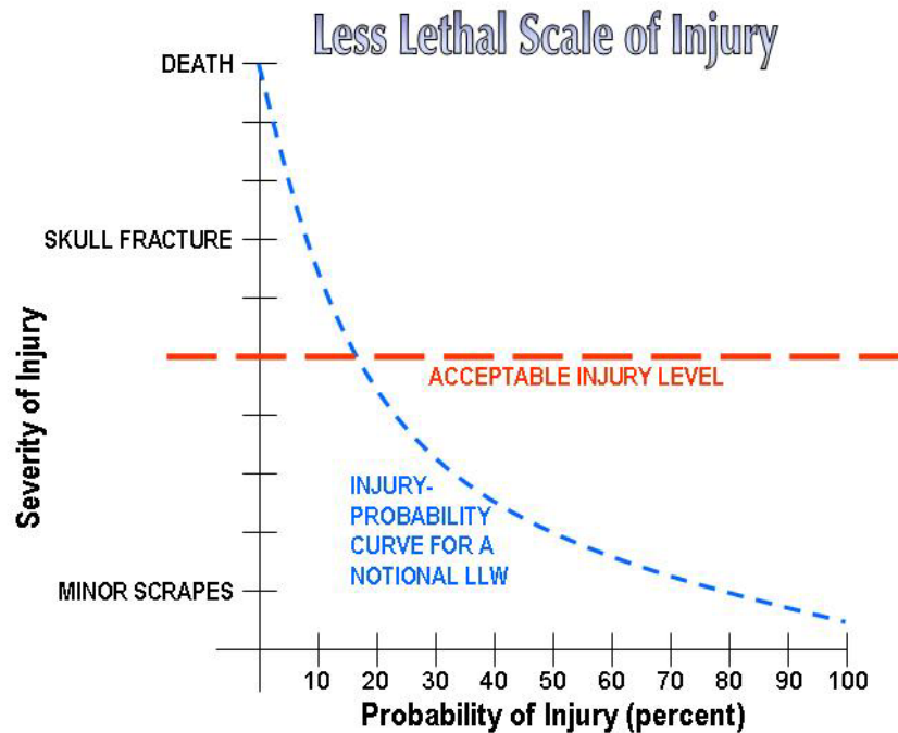
Figure 2-1. Example of what a less-lethal weapon injury scale might look like. The area above the broken red line displays all unacceptable injury types. The area below the broken red line encompasses all of the acceptable injuries without considering probability. The curve represents a notional less-lethal weapon’s injury types and associated probabilities of occurrence.
