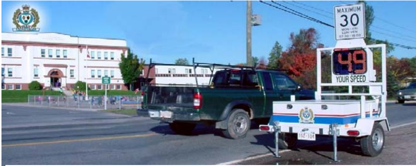
RADAR trailer set up on Canada Street in a marked school zone.
