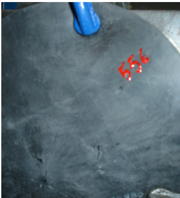
Figure 4.10: Target Type M - 5.56mm, 9mm and #4 Buck round, no complete penetration, Post Impact Front View
