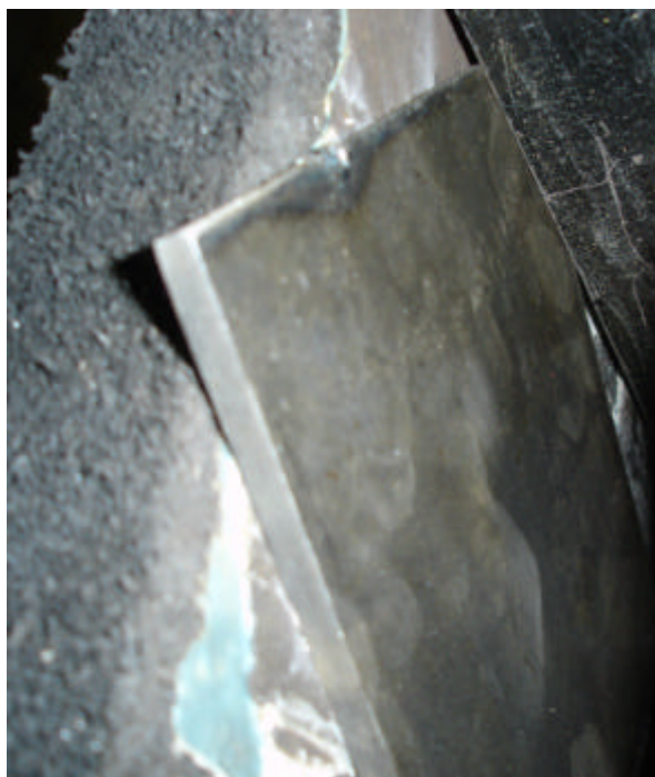
Figure 4.8: Target Type J - 5.56mm, 9mm and #4 Buck round, no penetration, Post Impact Front View
