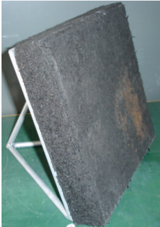
Figure 2.1: Alternative Target Type 1: Recycled Rubber with \frac{1}{4} " AR500 Steel backing
