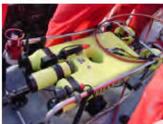
The Simrad imaging sonar can be seen mounted on the top left corner of the Phantom HD2 ROV frame.
