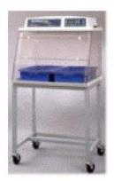
The unit meets O.S.H.A. standards for fume hood face velocity and ANSI Z9.5 standards for ductless fume hoods.
