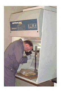
The AirClean Systems Forensics Workstation is an ideal unit for protecting the operator from toxic gases and particulate materials used in routine analysis. A modified IDENTIFICATION version is available to hold a macroviewer with camera stand. The unit protects the operator from residual isocyanoacrylate and aluminumbased powders used on exhibit materials. Other commonly used chemicals such as methanol are also contained.
