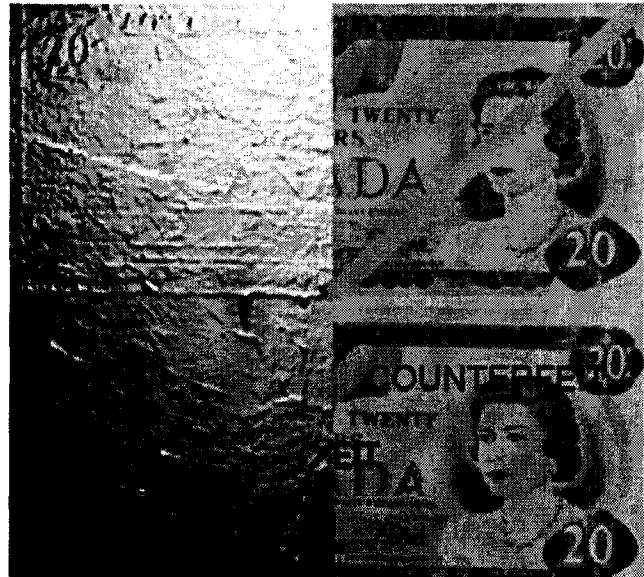
Figure 3: The left half is an Edge of Light image of genuine (top) and counterfeit Canadian $20 bank notes. Covering the notes with aluminum foil removes any non-topographical features from the image. The right half is a normal view of the same notes.
