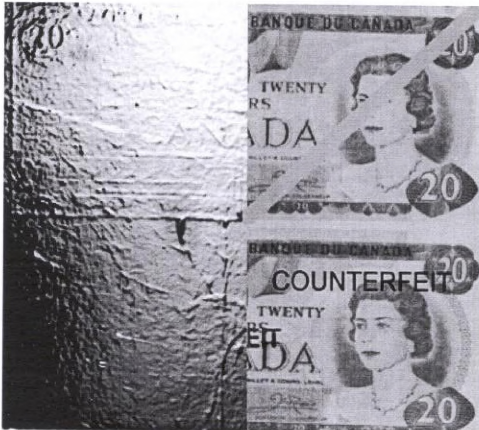
Figure 1: The left half is an Edge of Light image of genuine (top) and counterfeit Canadian $20 bank notes. Covering the notes with aluminum foil removes any non-topographical features from the image. The right half is a normal view of the same notes.
