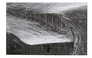
Ruger 10/22 Firing Pin Impression taken with the Scanning Electron Microscope
