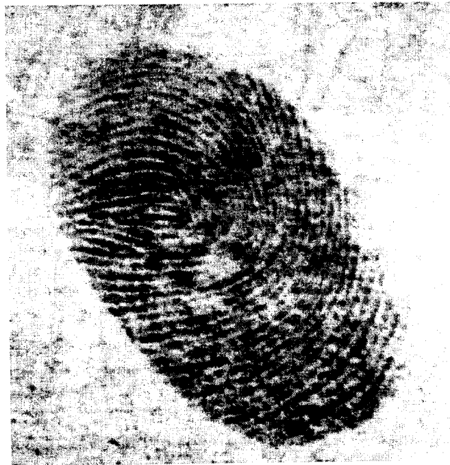
Figure 6. EOL scan of fingerprint on glass sheet (Note: Fingerprints are untreated).
