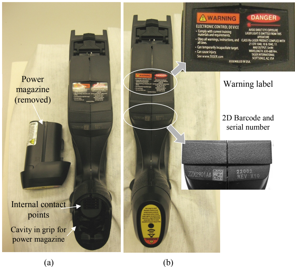
Figure 5: Taser X2 viewed from bottom (a) with power magazine removed and (b) with a power magazine inserted, with insets of the warning label, barcode, and serial numbers.
