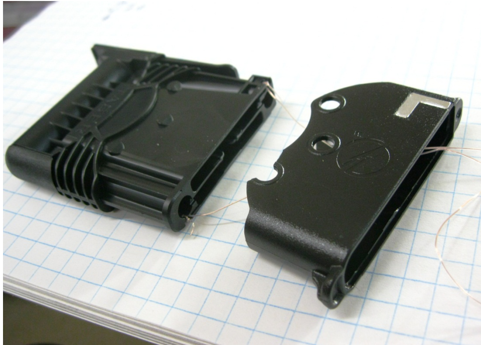
Figure 47: Taser X2 cartridge separated into two parts
