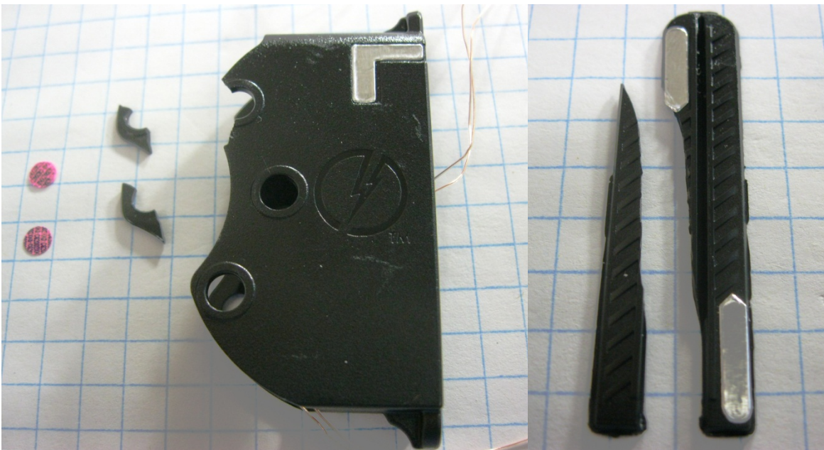
Figure 48: Side view of the hollow cartridge part (left) and the recovered blast doors (right)
