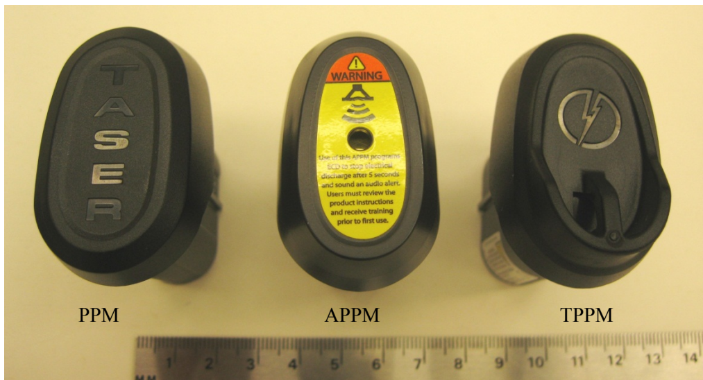
Figure 16: Three different Taser X2 PPM models viewed from the bottom
