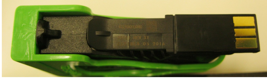
Figure 14: Smart Cartridge showing the three contact points and serial number
