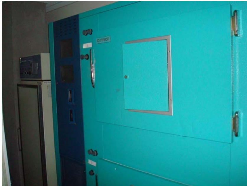
Figure 3 Conviron E7/2 plant environmental chamber
