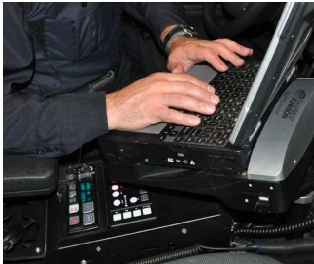
Figure 4: Computer partially blocks access to console
