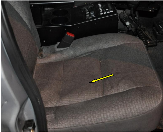
Figure 16: Seat foam, bottoming out
