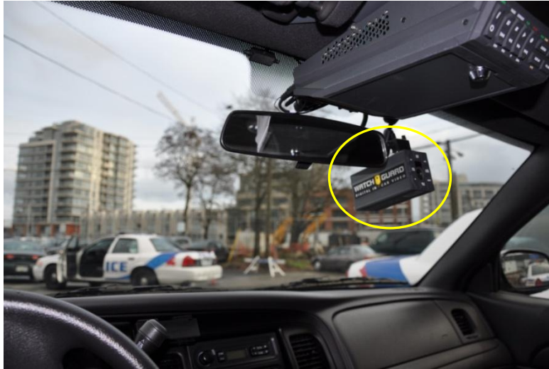
Figure 14: Above mirror lights and in-car camera in line of vision to traffic lights
