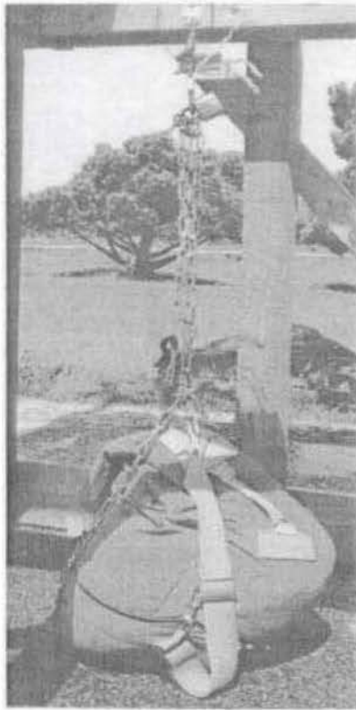
Photo 5. The “crash test dummy”, made of a burlap army bag, filled with sand.
