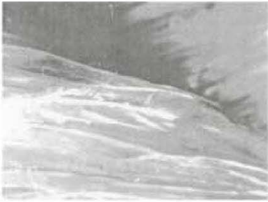
Photo 53. Filamentation and flattened fibre of drag trial ligature rope (20x).
